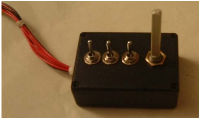
The Control Box Built and Wired Up
