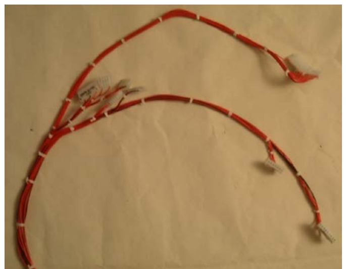
Take up the slack in the loom and tie the cables together. This is best done with the boards connected to the PCB's
