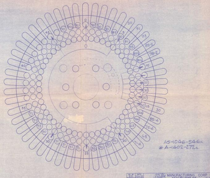
AFTER WIRING - WIRE BRUSH RIVET HEADS.
