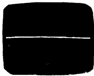
No Vertical Deflection
