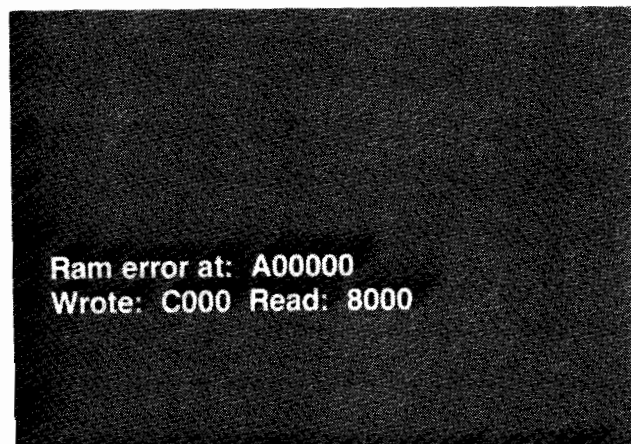
Figure 2-2 RAM Test Fails
