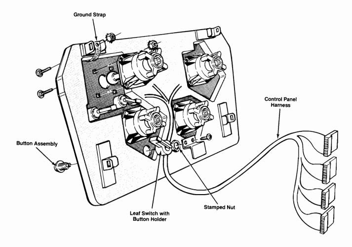
Figure 4-3 Pushbutton Leaf Switch Removal
