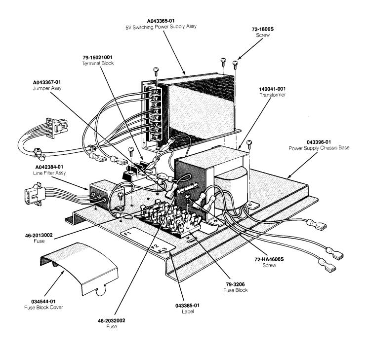
Figure 5-4 Switching/Linear (SL) Power Supply Assembly A043363-01 A
