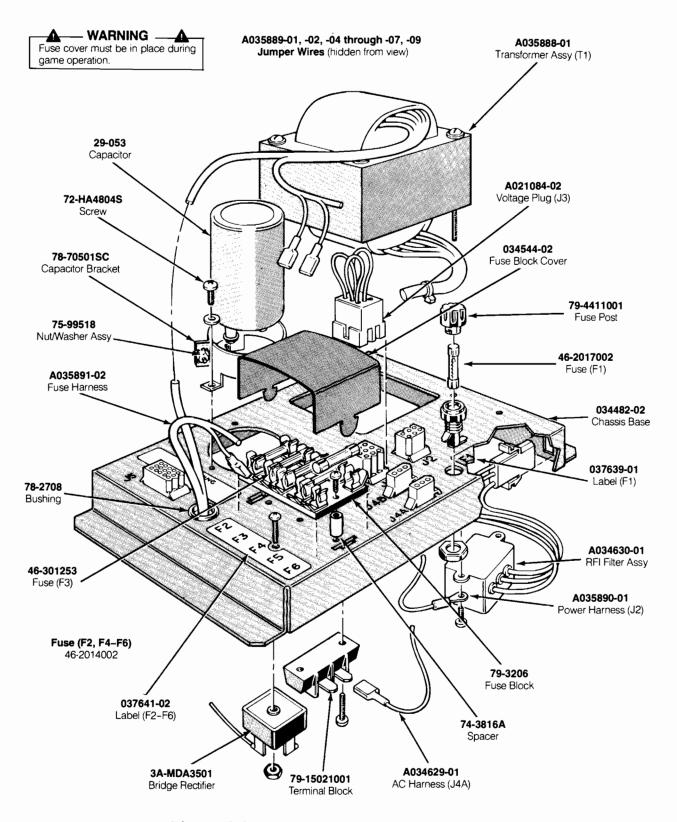
Figure 5-5 Linear Power Supply Assembly A037671-18 N
