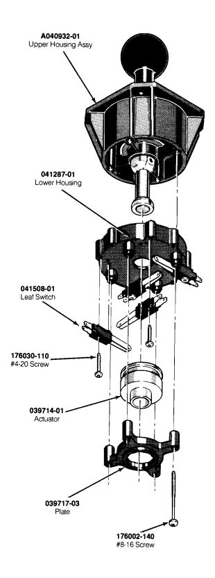
Figure 5-3 Joystick Assembly A040934-03 B
