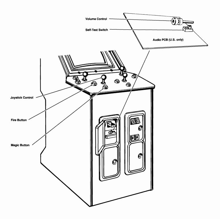
Figure 1-3 Control and Switch Locations
