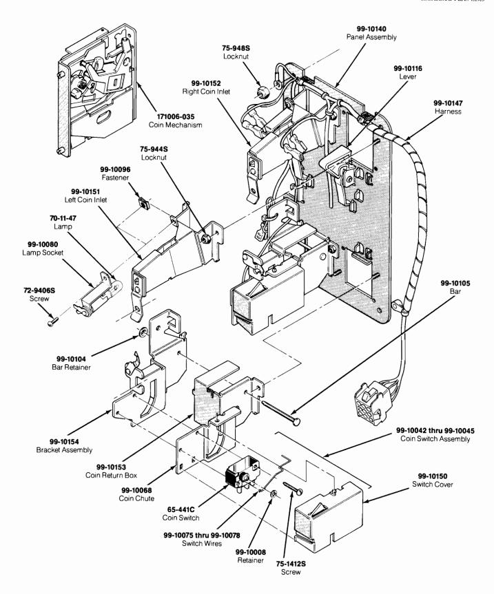
Figure 5-7 Coin Acceptors, Inc. Coin Door Assembly 171027-001 A
