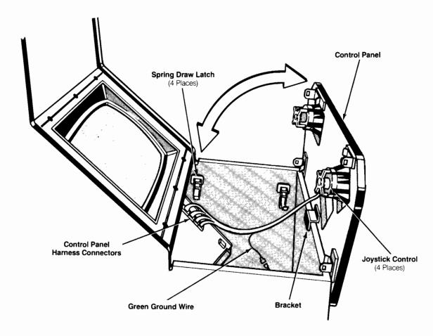
Figure 4-1 Control Panel Removal
