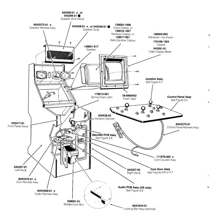
Figure 5-1 Cabinet-Mounted Assemblies A043350-01 and -51 D
