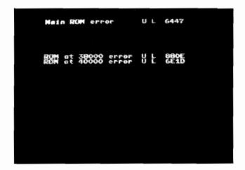
Figure 3-2 ROM Test Fails
