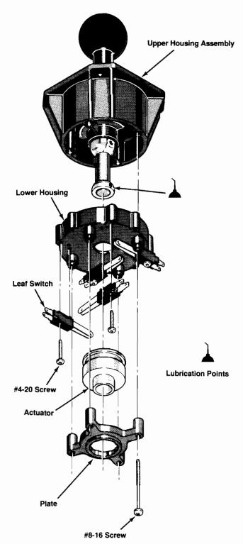
Figure 4-2 Joystick Lubrication
