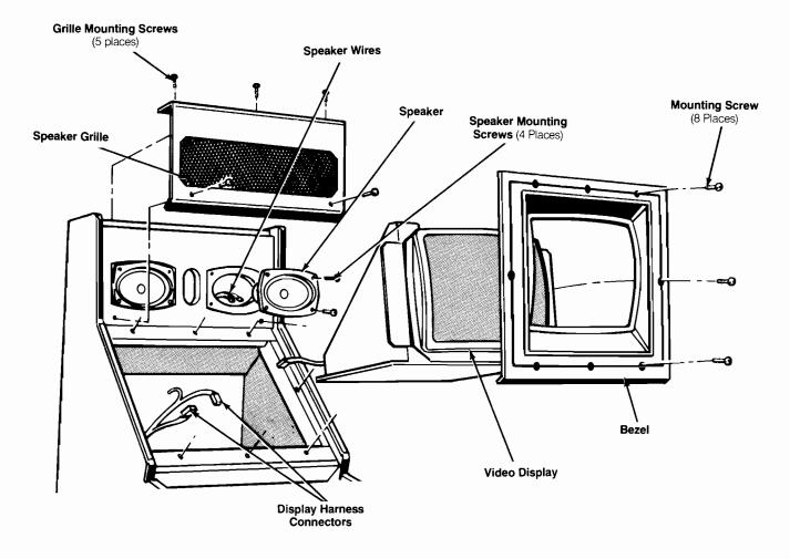
Figure 4-5 Video Display and Speaker Removal
