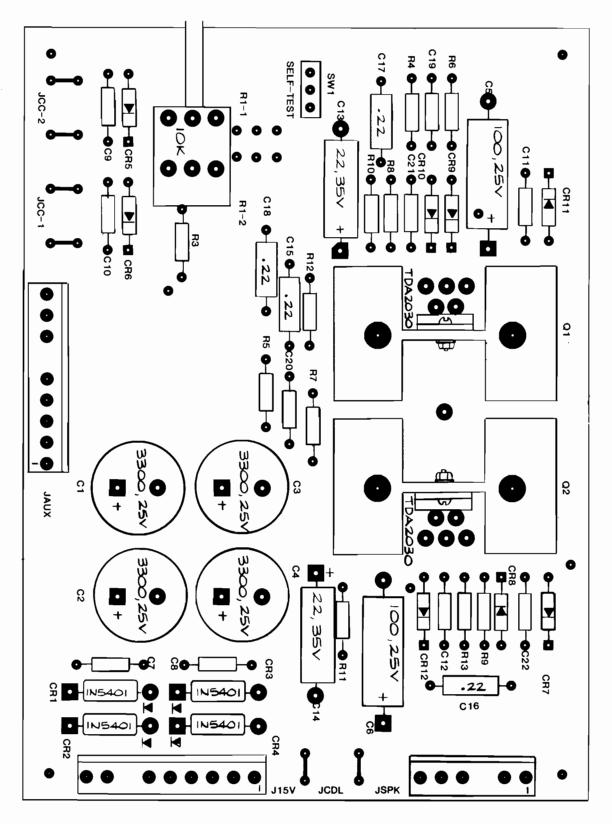
Figure 5-9 Audio PCB Assembly A043354-01 B
