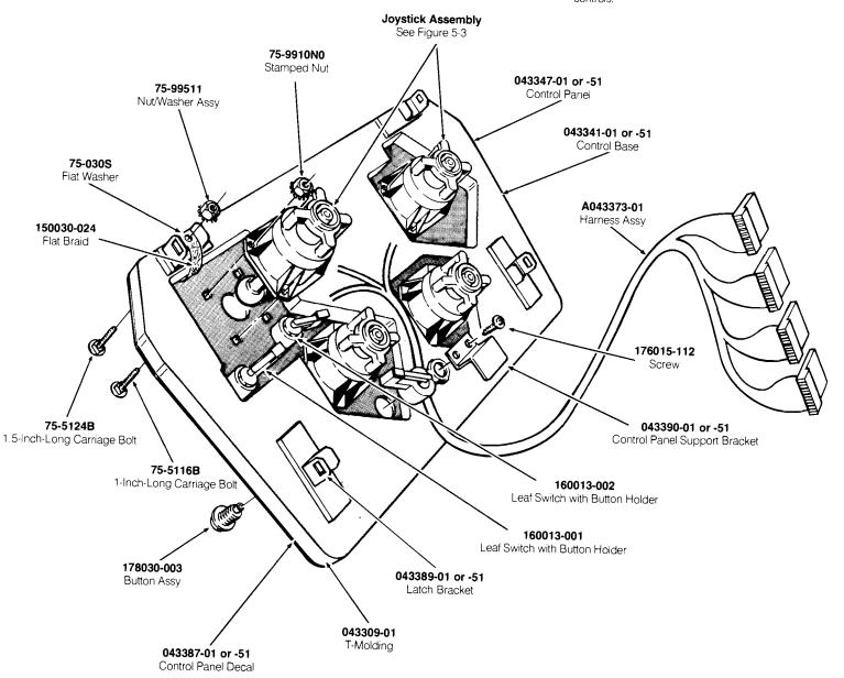
Figure 5-2 Control Panel Assembly A043386-01 B (U.S.) or A043386-51 B (Ireland)
